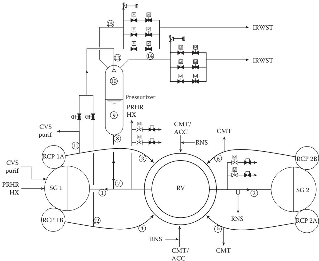
FIGURE 2.24 AP-1000 reactor coolant system schematic flow diagram.
